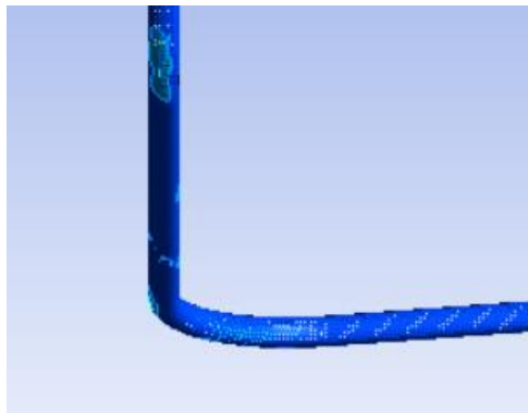
Gambar 2. kontur particle mass concentration diameter coal ash 840 \mu\text{m}
