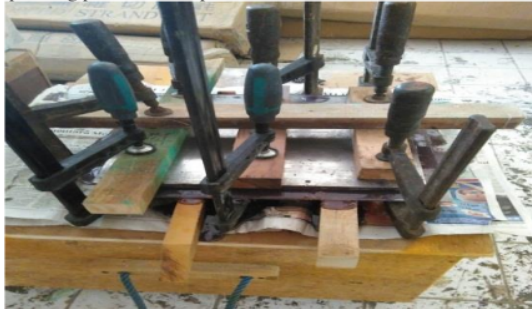
Fig 2. The process of making particle board
