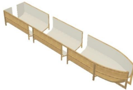
Figure 2 Multi-mold design of single hull shape
