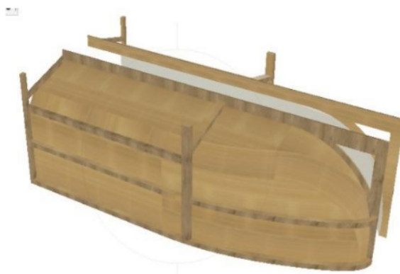
Figure 6 Fore Part Mold
